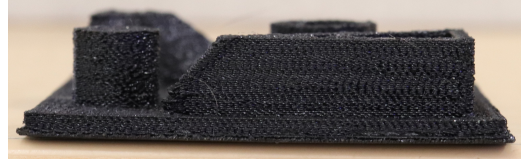
(b) 0.13 g vibration at 40.7 Hz. No isolation. Ra roughness: 946.15 \mu\text{in} .
